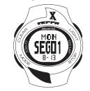
Once a segment is selected, press LAP button E to view the contents of that specific segment. The display will show the lap number on the top row, the lap time on the middle row and the total elapsed time will appear on the bottom row.
